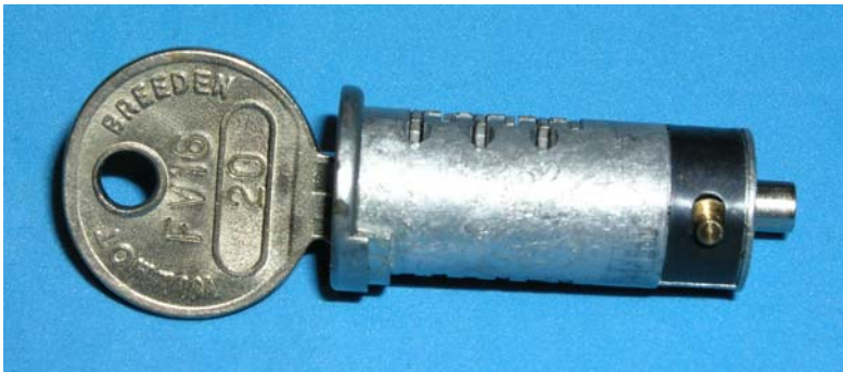
LOCK BARREL WITH KEY NOTE BRASS PIN AND LOCK RETAINING PIN AT END ALL BLADES MUST BE DOWN EVEN WITH THE BARREL TO INSTALL THE BARREL
